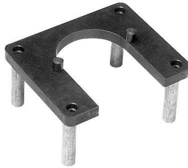
Figure 6 Main holding tool (horse hole): Code No.: SJ 151-9000-1.
