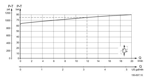
The pressure relief valve protects the pump and steering unit against excess pressure and limits the system pressure while steering.
