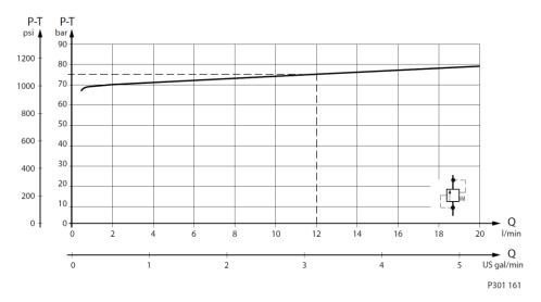
The pilot pressure relief valve together with the priority valve limits the maximum steering pressure P-T. The pilot pressure relief valve is set at an oil flow to the priority valve of 12 l/min [3.17 US gal/min]. For the OSPM LS load sensing dynamic steering units, the setting values are valid at a dynamic flow of 0.6 l/min [0.16 US gal/min].
