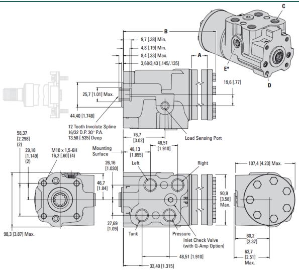
Figure 39 20 Series Installation Drawing
