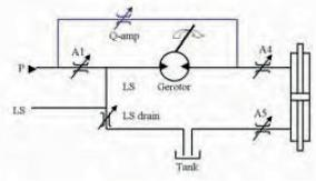
Figure 23 Flow Amplification without Cylinder Damping
