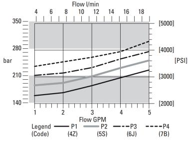
Figure 42 Cylinder Relief Valve Pressure
