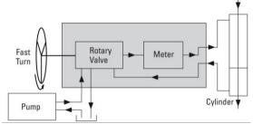
Figure 17 Conventional Steering Control Unit
