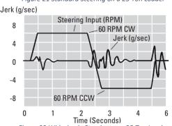
Figure 22 Wide Angle Steering on a 25 Ton Loader
