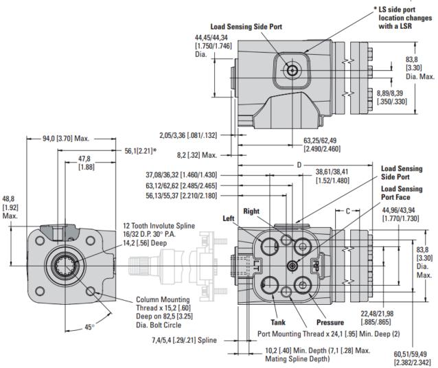
Figure 31 Installation Drawing
