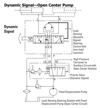
Figure 6 Dynamic Signal—Open Center Pump
