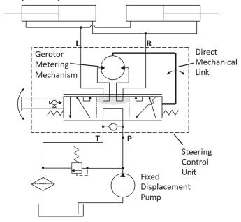
Figure 10 Open Center System Load Reaction Circuit
