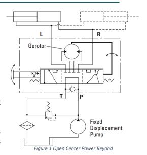
Since steering has priority, all flow, if required, will be di-verted to steering. The tank port of the steering unit has flow only when steering is operated. Thus, flow out of the auxiliary ("PB") port and the tank port will fluctuate or stop depending on steering input.
