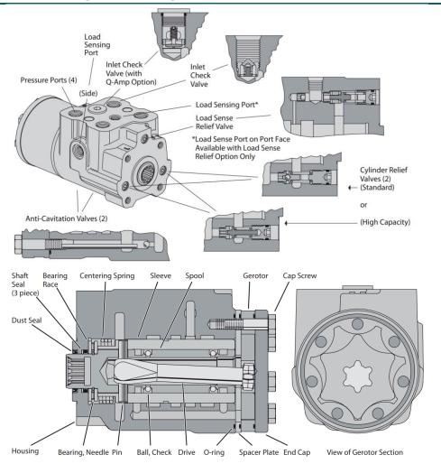
Figure 41 Sectional Drawing and Integral Valves
