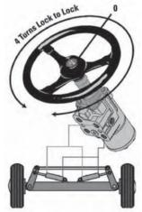
Figure 27 Traditional Metered Steering
