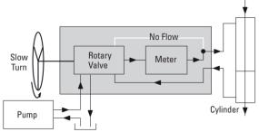
Figure 19 Q-Amp Steering Control Unit – Slow Turn
