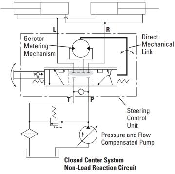
Figure 9 Closed Center System (Non-Load Reaction Circuit)
