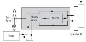
Figure 18 Q-Amp Steering Control Unit – Fast Turn
