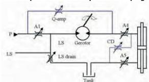
Figure 24 Flow Amplification with Cylinder Damping
