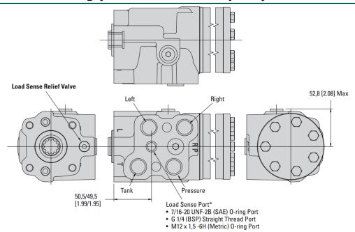
\*Load sense port on port face (is only available on units with load sense relief valve).
