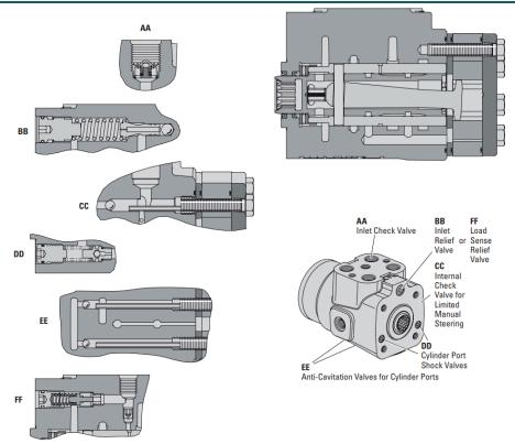
Figure 32 Sectional Drawing and Integral Valves
