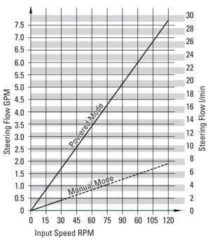
Flow vs RPM (for each operating mode)
