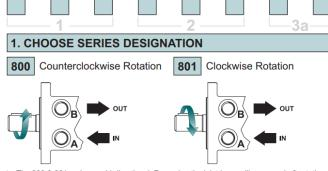
▶ The 800 & 801 series are bi-directional. Reversing the inlet hose will reverse shaft rotation.
