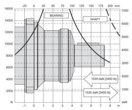
Figure 53 Wheel Mounts Allowable shaft load/bearing curve
