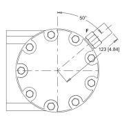
E: 10 Series/2-Way Valve Cavity 7/8-14 UNF F: Valve Cartridge Installed
