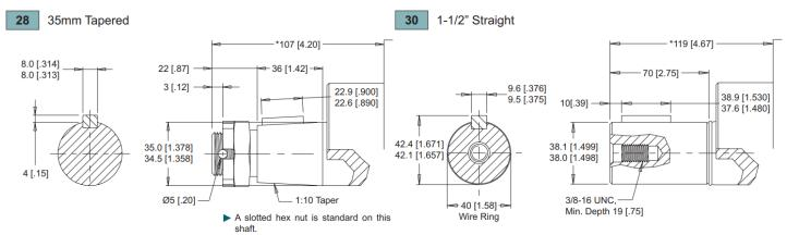
Max. Torque: 1200 Nm [10600 lb-in] Max. Torque: 1200 Nm [10600 lb-in]
