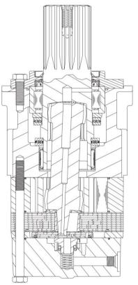
Figure 37 DT 700 Hydraulic Motor Standard
