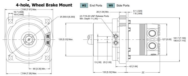
Figure 24 DR 610 Series, 4-hole Wheel Brake Mount
