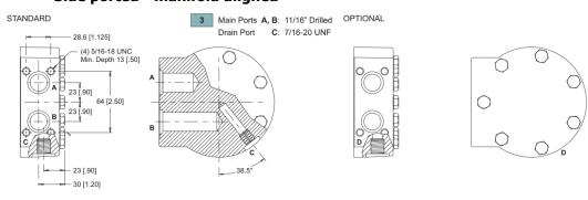
Figure 17 DR Porting (manifold aligned)
