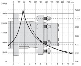
Figure 46 DT 740 Wheel Hub Mounts
