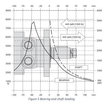
Example load rating for mechanically retained needle roller bearings
