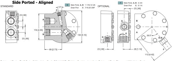
D: Internal Drain E: 10 Series/2-Way Valve Cavity 7/8-14 UNF F: Valve Cartridge Installed G: Internal Drain Placement With Valve Cavity Figure 42 DT Porting (Side Ported - Aligned)
