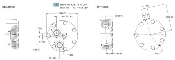
D: Internal Drain E: 10 Series/2-Way Valve Cavity 7/8-14 UNF F: Valve Cartridge Installed
