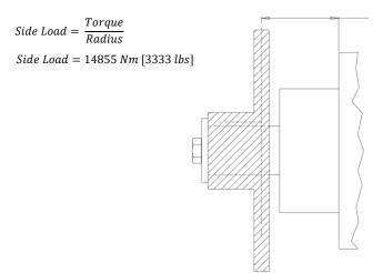
Figure 7 Induced side load
