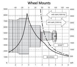
Figure 22 Magneto & SAE A Mounts Allowable Shaft Load / Bearing Curve
