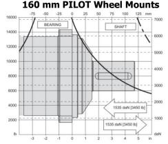
Figure 52 160 mm PILOT Wheel Mounts Allowable shaft load/ bearing curve
