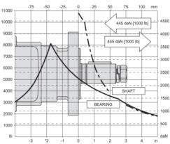
Figure 28 DR 620 Allowable Shaft Load/ Bearing Curve
