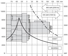
Figure 44 SAE C Mounts Allowable Shaft Load / Bearing Curve
