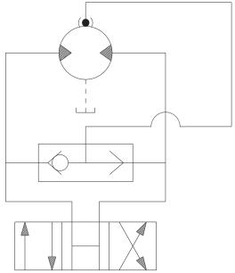
Figure 1 Typical Motor/ Brake schematic
