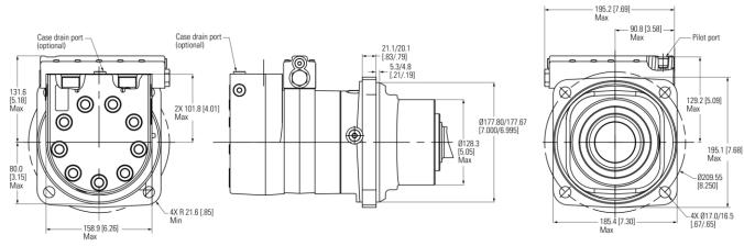
Figure 37 Two speed wheel mount open loop
