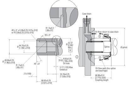
Figure 21 Install instruction bearingless mount
