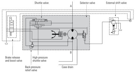
Figure 45 Two speed brake motor circuit
