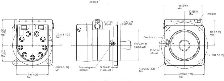
Figure 38 Two speed bearingless closed loop
