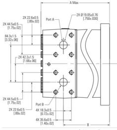
Figure 14 Wheel Mount manifold interface
