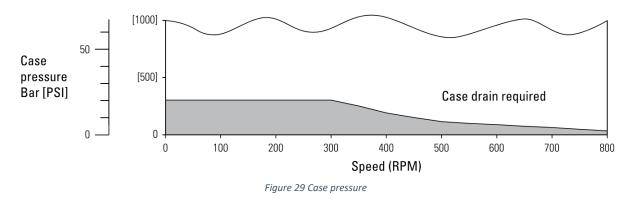
**Note**: Use of a case drain is optional in an open loop circuit if motor case pressure does not exceed 300 psi.
