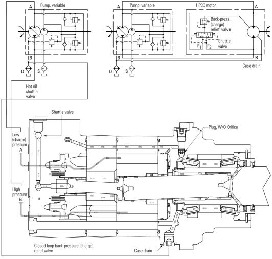
Figure 41 Closed loop circuit
