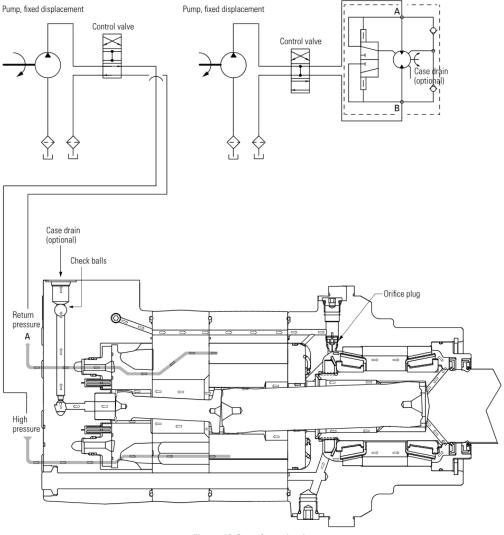
Figure 43 Open loop circuit
