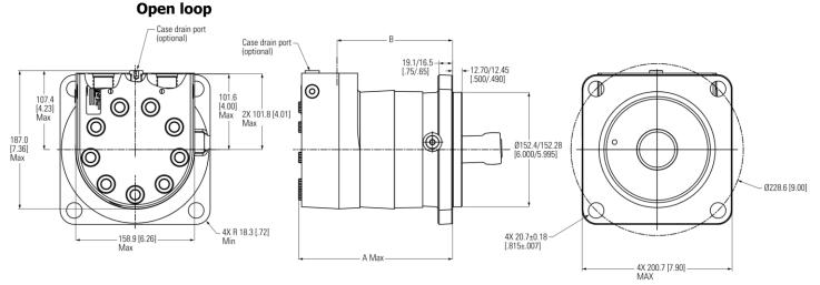
Figure 20 Bearingless mount open loop
