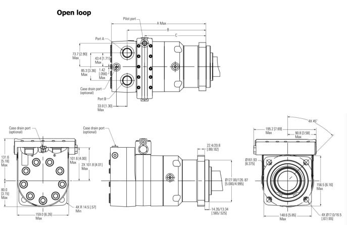
Figure 34 Two speed standard open loop
