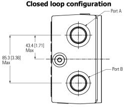
Figure 17 Bearingless mount closed loop configuration
