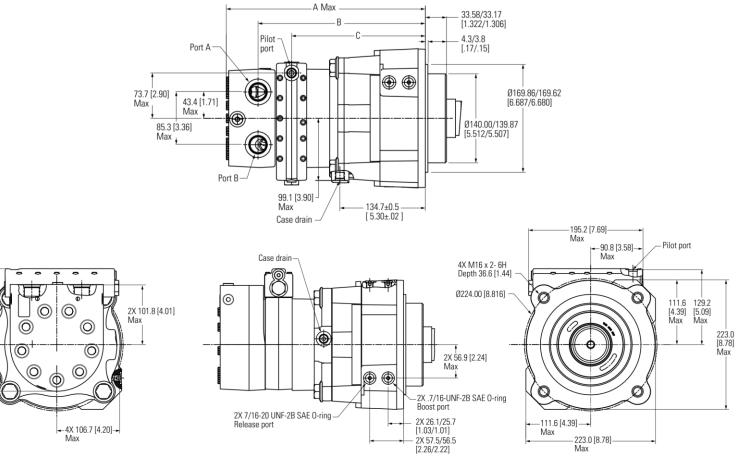
Figure 48 Brake motor two speed closed loop
