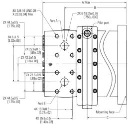
Figure 35 Two speed wheel mount manifold interface
