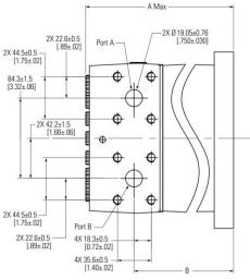
Figure 11 Standard mount Manifold Interface
