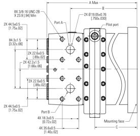
Figure 31 Two-speed standard motor manifold interface
