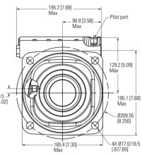
Figure 36 Two speed motor wheel mount closed loop
