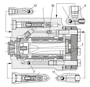
Figure 1: Cross Section LAGU
