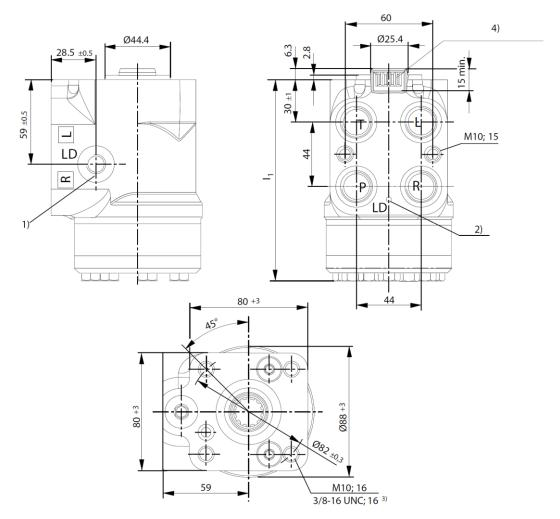
Figure 17: Dimensions for LAGU and LAGU LD & LDA versions (in mm)
