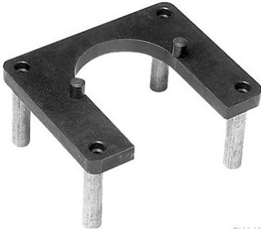
Figure 6 Main holding tool (horseshoe): Code No.: SJ 151-9000-1.
