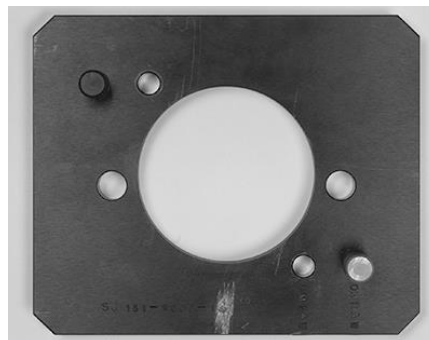
Figure 10 Holding tool for OMPW N Code No.: SJ 151-9000-14
