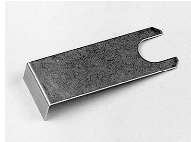
Figure 7 Fork. For use when fitting OMP cardan shaft Code No.: SJ 151-9000-3.
