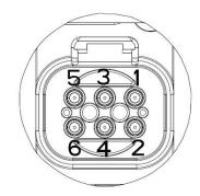
Figure 10: Connector Deutsch DT14-6P
